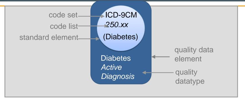
Standard element (including code set and code list) as part of the quality data element (rounded rectangle). The standard element (light blue circle) has a *code set* and specific *code list* and is part of the quality data element. The color of the circle indicates the standard category, in this example diagnosis.
